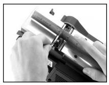
Figure 10. Setting cutter height.
